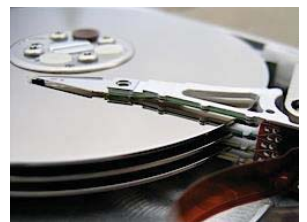
Hard drive read/write head
